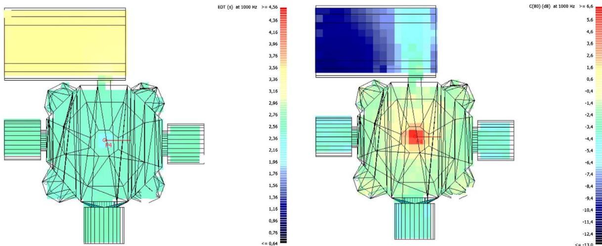
**Figure 7.** Spatial distribution of simulated EDT (left) and  $C_{80}$  (right) values at 1000 Hz considering an omnidirectional sound source at the centre of the octagonal hall (Odeon).
