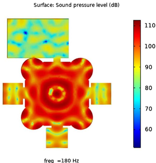
**Figure 5.** Simulated sound pressure level (dB) distribution at 180 Hz considering a *Monopole point source* at the centre of the octagonal hall (COMSOL).
