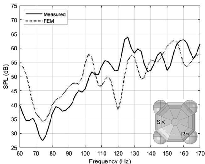
**Figure 4.** Comparison between measured and simulated frequency responses corresponding to the source-receiver pair shown at bottom right (COMSOL).
