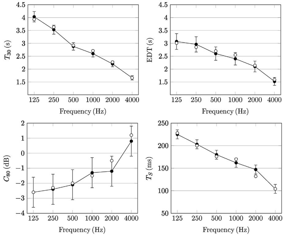
**Figure 6.** Calibration results: comparison between experimental data (black) and numerical simulations (white) through GA techniques (Odeon). Values have been averaged over all the receivers in the main octagonal hall and refer to sound source S1 (see Fig. 2).
