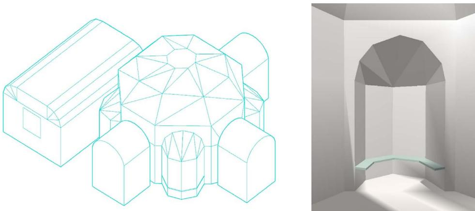
**Figure 3.** Views of the 3D virtual model of the central octagonal hall ( $220 \text{ m}^3$ ) surrounded by the adjacent halls ( $130 \text{ m}^3$ ) in Odeo Cornaro's building (overall 350 surfaces approximately): outside and inside views (Sketchup).
