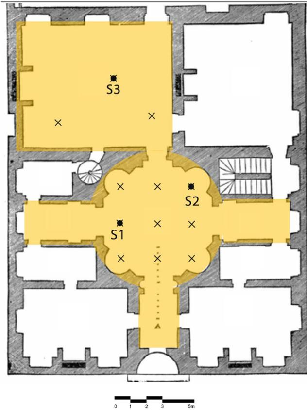
**Figure 2.** Plan of the Odeo Cornaro with the sound source (S1, S1, and S3) and receiver locations (x) employed during the acoustic measurements.
